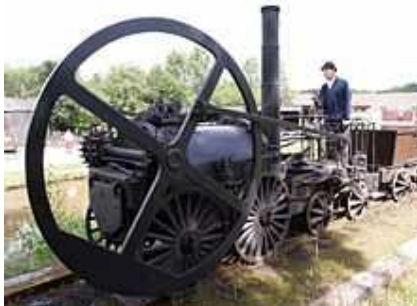
Figure 1 Flywheel to Even Out the Power of Its Single Cylinder.
