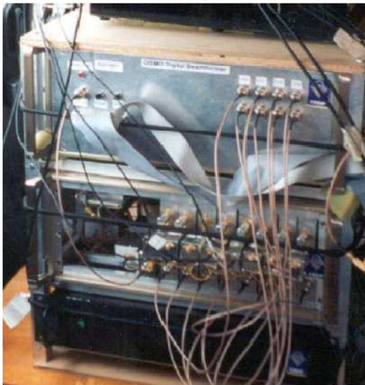
Figure 6: Technology demonstrator implementing a spatial null steering algorithm
