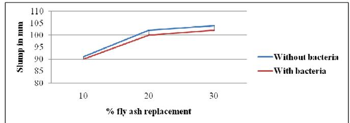
Figure 5 Variation of slump for M40 grade concrete
