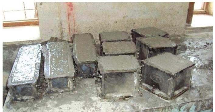
Figure 6 Moulds of cement concrete cubes being casted in the Laboratory
