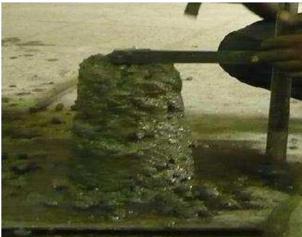
Figure 2 Slump of concrete being measured in Laboratory.
