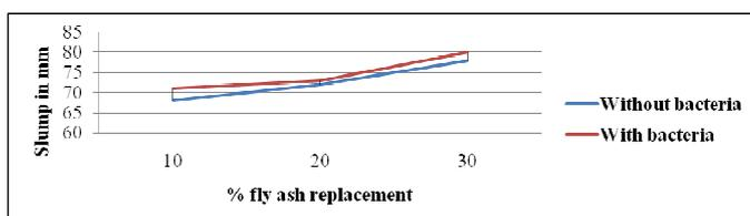
Figure 3 Variation of slump for M20 grade concrete
