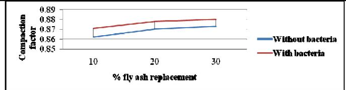
Figure 4 Variation of compaction factor for M20 grade concrete.
