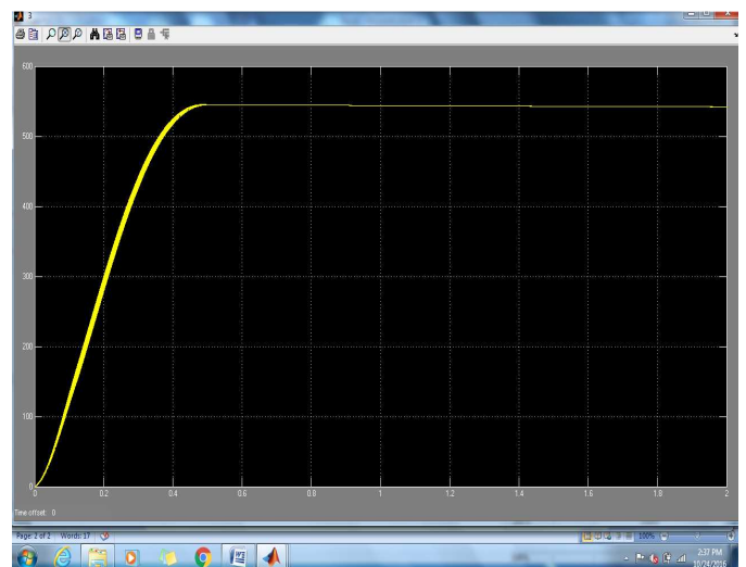
Fig.11. Boost Converter Voltage at PV side.
