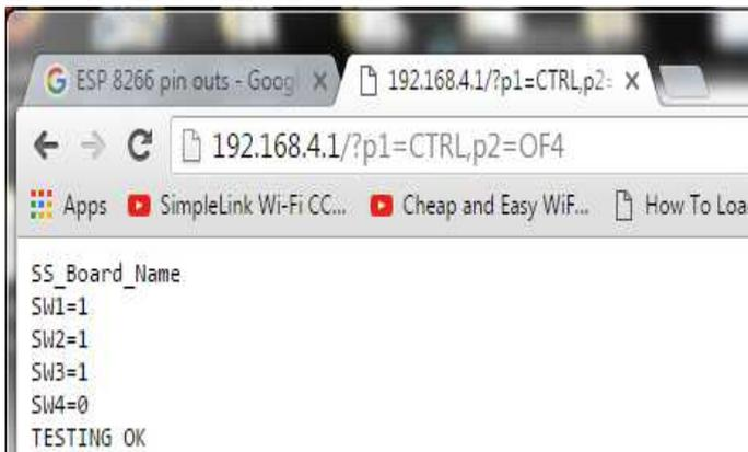
Figure 3.7: Result Switch 4 OFF
