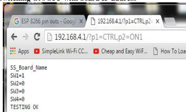
Figure 3.3: Result Switch 1 ON
