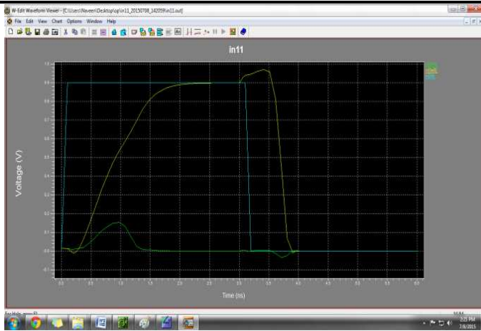
Fig.5: Simulation of Inverter based amplifier design
