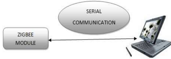
Fig2: Control section/server section
