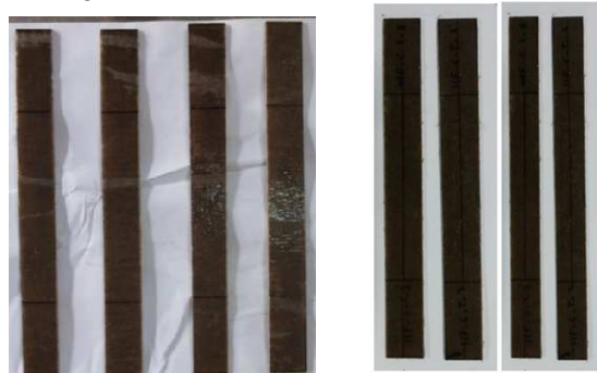
Fig 3.2. Hemp-epoxy samples before tensile testing
