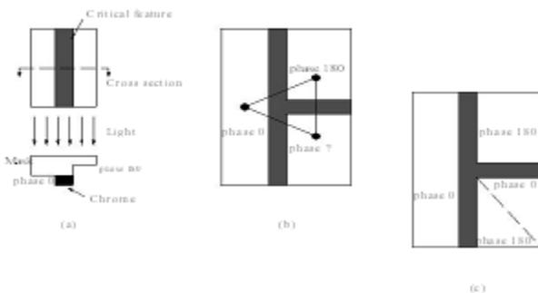
Fig. 2. (a) Alternating Phase Shifting Mask(Alt-PSM). (b) Phase conflict occurs for a T-shaped critical feature. (c) Phase conflict removal by splitting a phase region.
