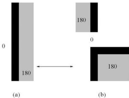
Fig. 6. Standard cell Alt-PSM composability.
