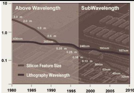
Fig. 1. Technology trend for transistor feature size
