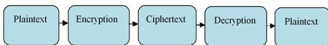
Fig1 The process of Encryption transforms Plaintext into Ciphertext and the process of Decryption transform Ciphertext into Plaintext.
