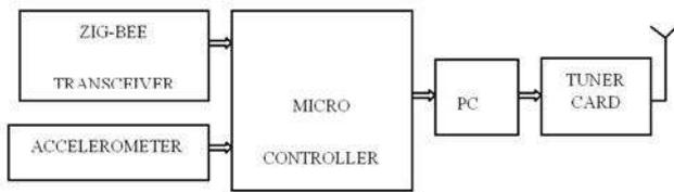
Fig. 4. Architecture of System Terminal Unit
