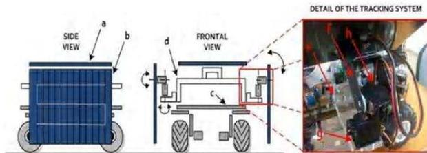
Fig. 5. Mechanical design of the solar tracking system of VANTER: (a) upper solar panel, (b) mobile solar panels, (c) aluminium chassis, (d) methacrylate chassis, (e) methacrylate support, (f) pan and tilt unit, (g) pitch servometer, and (h) yaw servomotor
