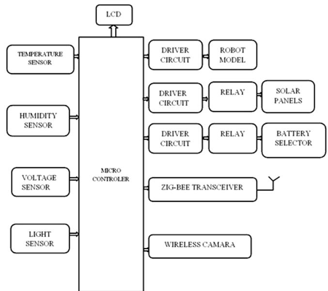
Fig. 3. Architecture of Robot terminal unit
