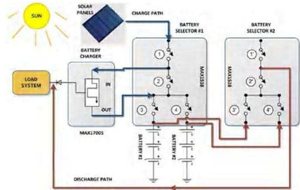
Fig. 6. Overall connection diagram for battery selectors
