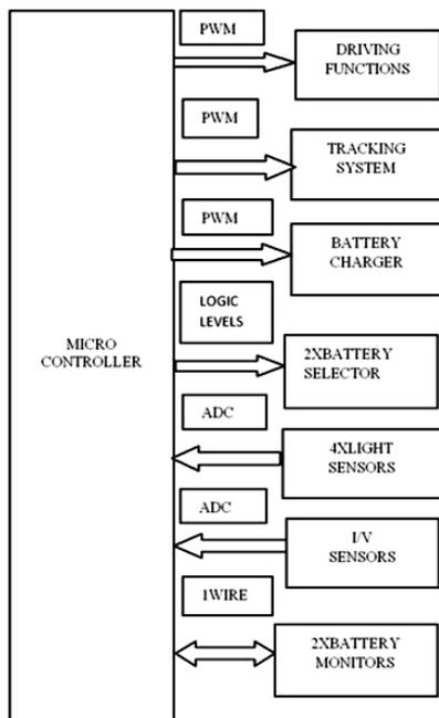
Fig. 2. Block diagram of the hardware architecture for VANTER.
