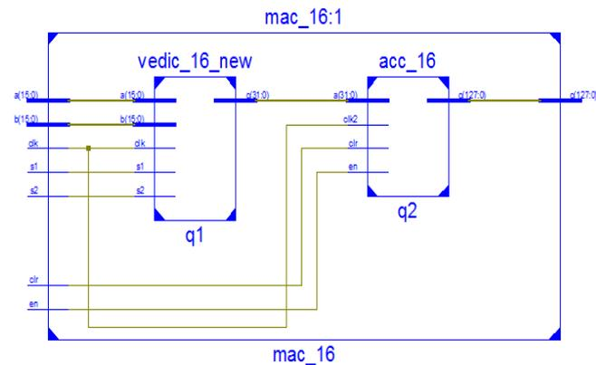
Fig 5.RTL schematic for 16-bit MAC using Mux. Simulated waveforms for 32-bit:
