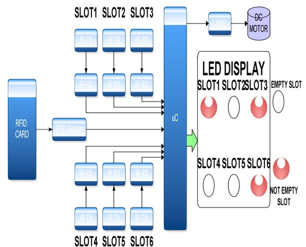
Block diagram of automated car parking using RFID
