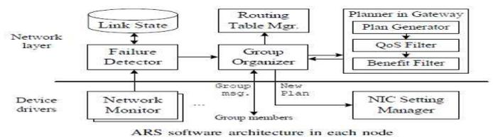
Fig 2: ARS is implemented across network and link layers as a loadable module of Linux 2.6 kernel.
