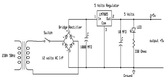
Fig 3.3.3 Circuit diagram of Regulated Power Supply with Led connection
