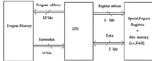
Fig.3.3. Architecture of PIC microcontroller
