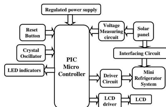
FIG 3.1: Block diagram of microcontroller based refrigerator control system
