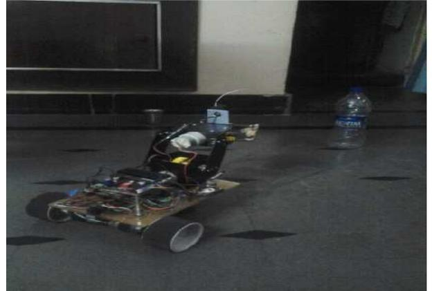
Figure 4.5 Wireless camera mounted on Robot
