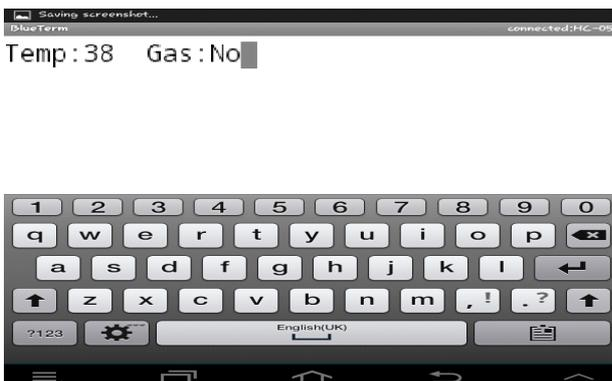
Figure 4.4 Displaying of temperature and gas parameters on mobile.
