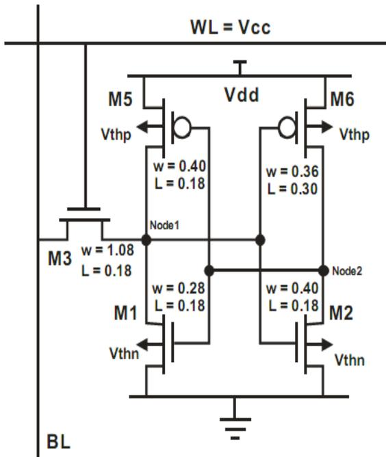
Fig 1. Block diagram of 5T SRAM CELL
