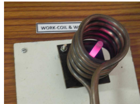
Figure 4 Work Coil and Work Piece At temperature 650 0 c the Iron Rod becomes Red Hot.
