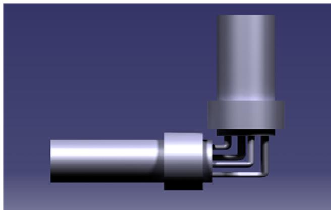
Fig.2 L-Pin Coupling (Top view)
