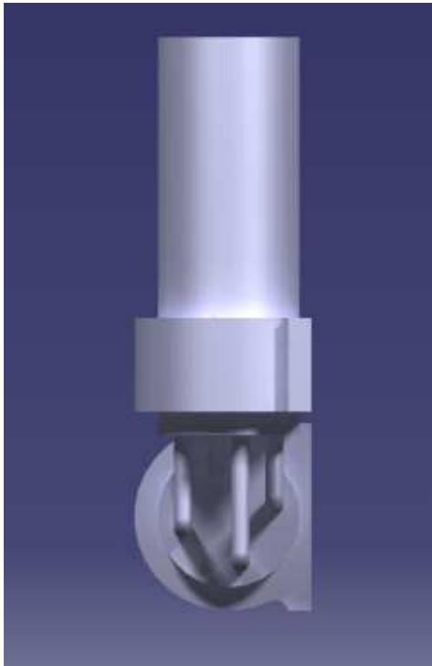
Fig.3 L-Pin Coupling (Side view)
