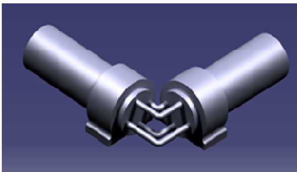
Fig.10 Final Assembly of L-Pin Coupling
