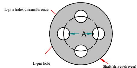
Fig.12 Side view of the Shaft (driver/ driven)
