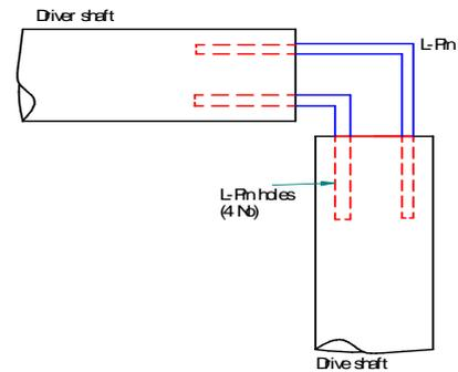
Fig. 11 Orthographic views of L-Pin Coupling
