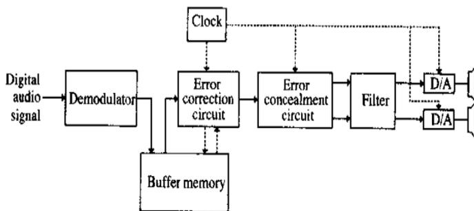
Fig.5 Block diagram of signal processing part of CD player
