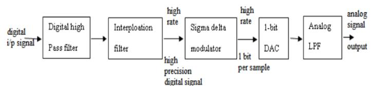
Fig.1 sigma-delta digital to analog converter
