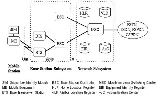
Fig.5 Block Diagram Of GSM
