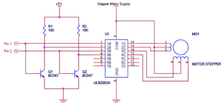
Fig.4 Wire Connection Of Unipolar Stepper Motor
