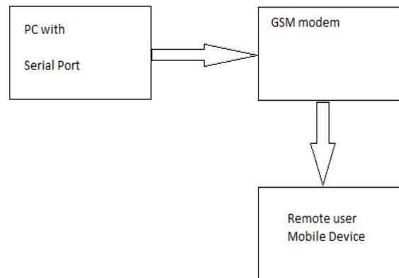
Fig.6 Block Diagram Of GSM Modem
