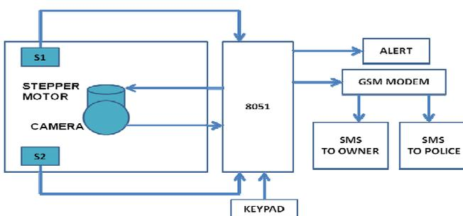
Fig.1 Block Diagram of Invisible Eye
