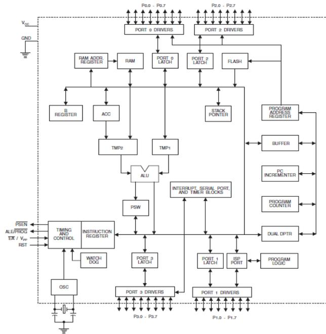
Fig.3 Block Diagram of Microcontroller
