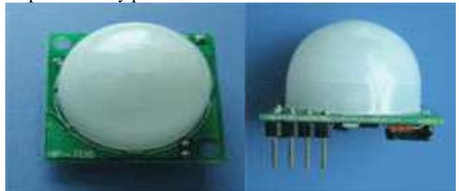
Fig.2 Motion detector module uses a motion detector IC and PCB mounted Fresnel lens.
