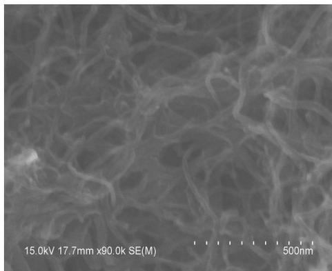
Fig. 1: SEM image of PMWCNT
