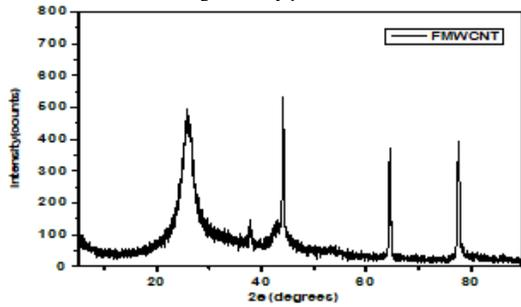
Fig. 7: X ray pattern of FMWCNT
