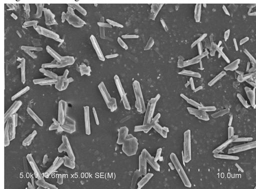
Fig. 5: SEM Image of 3% FMWCN innafion membrane
