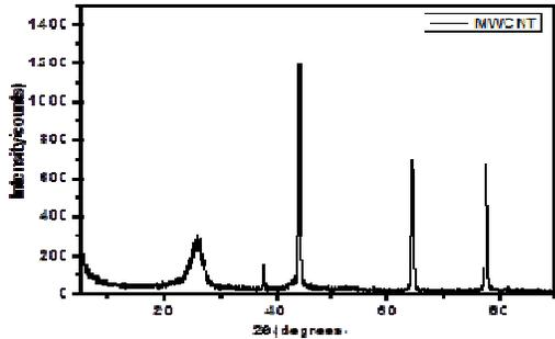
Fig. 6: X ray pattern of MWCNT
