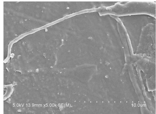
Fig. 3: SEM Image of 1% FMWCN innafion membrane
