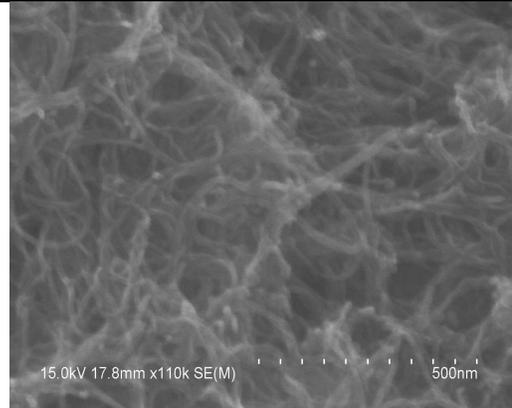
Fig. 2: SEM image of FMWCNT
