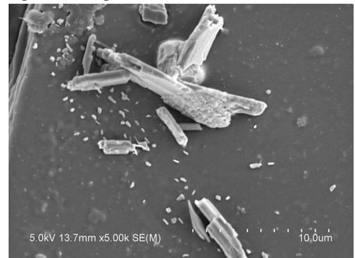
Fig. 4: SEM Image of 2% FMWCN innafion membrane
