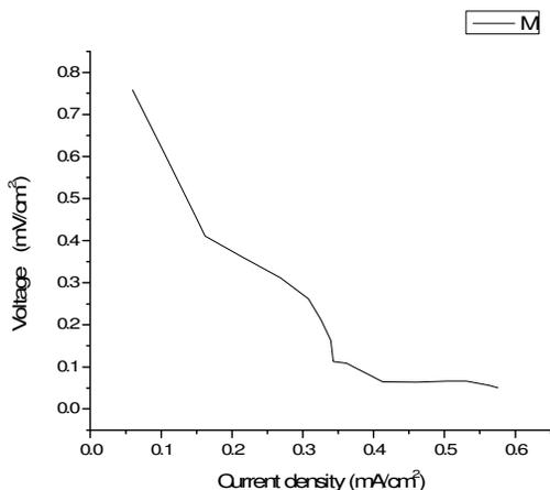
Fig. 10: I-V curve of MWCNT
