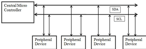
Fig 1.6 Block diagram of Inter-Integrated Circuit protocol
