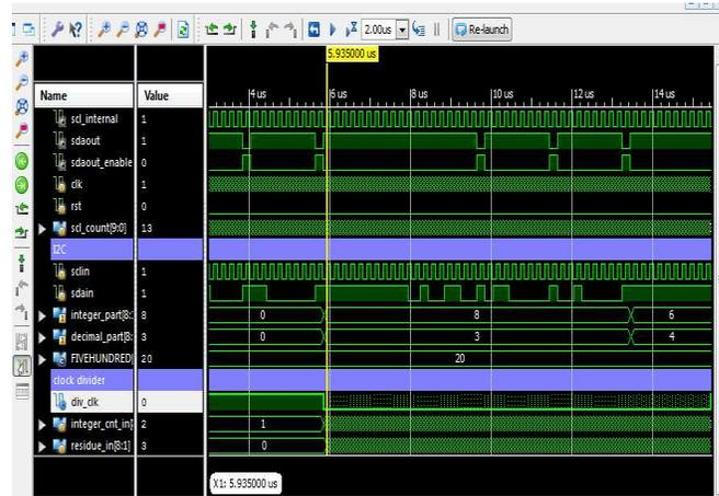
Fig 5.1SIMULATION RESULTS OF CLOCK DIVIDER (XILINX ISE SIMULATOR)
