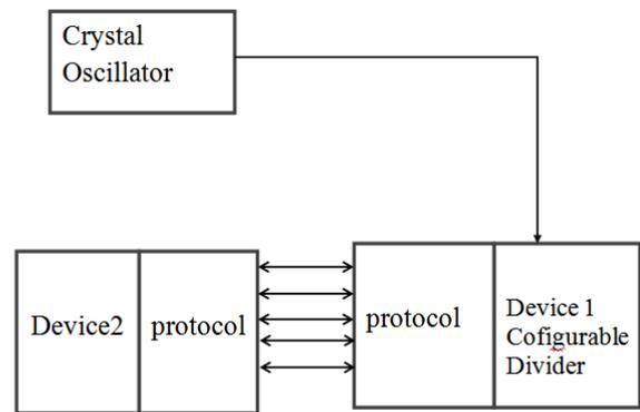
Fig.1.4 Block diagram of frequency divider
