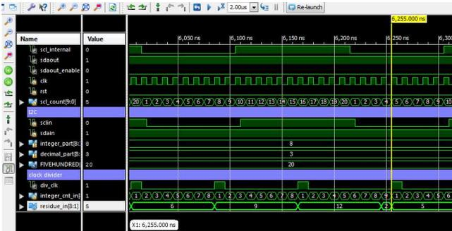
Fig:5.4 SIMULATION RESULTS OF CLOCK DIVIDER (XILINX ISE SIMULATOR)
