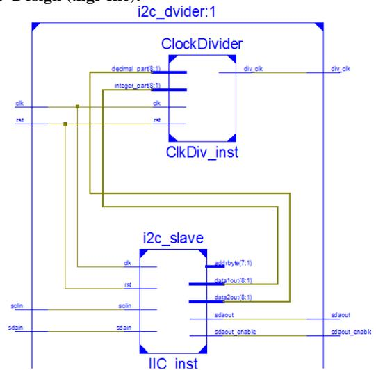
Fig 5.5 I2c divider block diagram
