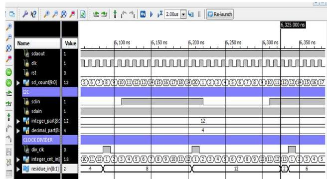
Fig:5.2 SIMULATION RESULTS OF CLOCK DIVIDER (XILINX ISE SIMULATOR)
