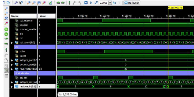
Fig:5.4 SIMULATION RESULTS OF CLOCK DIVIDER (XILINX ISE SIMULATOR)
