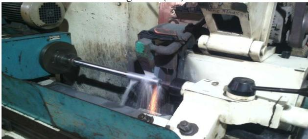
Fig.1 Cylindrical Grinding Process on test specimen
