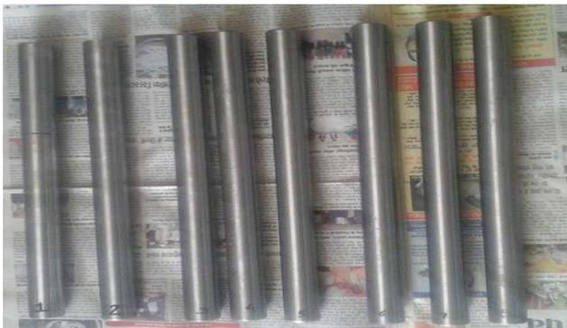
Fig. 2 Work pieces after cylindrical Grinding Process
