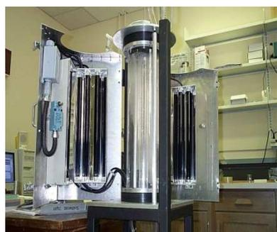
**Figure 1: Photo Catalytic Reactor**
