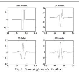
Wavelet Transform is used to split the signal into a bunch of signals and represents the same signal, but all corresponding to different frequency bands. The principle advantage is they provide what frequency bands exists at what time intervals. Wavelet transform of any function f at frequency a & time b is computed by correlating f with wavelet atom as
