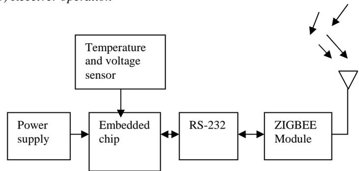
Fig.2 Block diagram of Receiver
