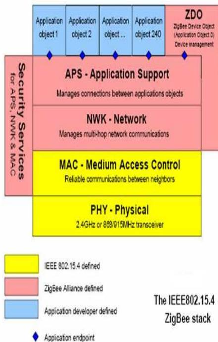
Fig 3: ZIGBEE stack
