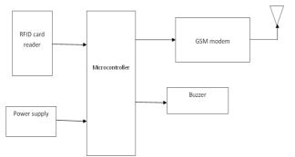
GSM modem is connected to the box containing question papers along with the microcontroller. Mobile of
