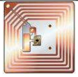
The amount of data storage on a tag can vary, ranging from 16 bits on the low end to as much as several thousand bits on the high end. Of course, the greater the storage capacity, the higher the price per tag.
