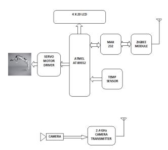
This system is a remote controlled Robotic arm system for surgery. The remote control media used is the regular Zigbee RF module. The system installed at the operation theater along with wireless camera, and receiver is placed at control room.
