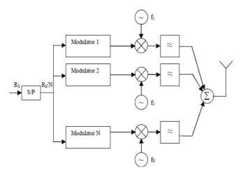
Figure 2.1: Block diagram of Generic MCM Transmitter
