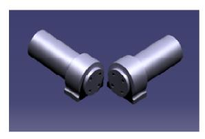
Fig.9 Shaft and Bearing Positioning
