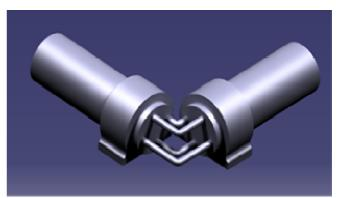
Fig.1 L-Pin Coupling (Isometric view)
