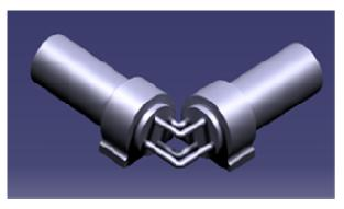
Fig.10 Final Assembly of L-Pin Coupling
