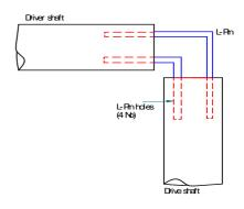
Fig. 11 Orthographic views of L-Pin Coupling
