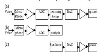
Fig. 1. Shows the process of digital processing of three types of audio signal. Part(a) represents a complete digital audio processing comprising (from left to right) a microphone, amplifier, ADC, digital processing material, DAC, amplifying section and speaker; an audio recognition system in (b), and a set of audio synthesis(c).
