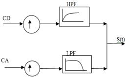
Fig 4: single level wavelet reconstruction(synthesis)
