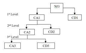
Fig 5: Three level wavelet decomposition tree.
