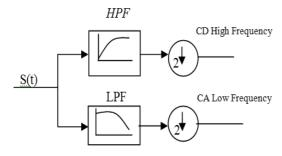
Fig 3.:single level wavelet decomposition(analysis).
