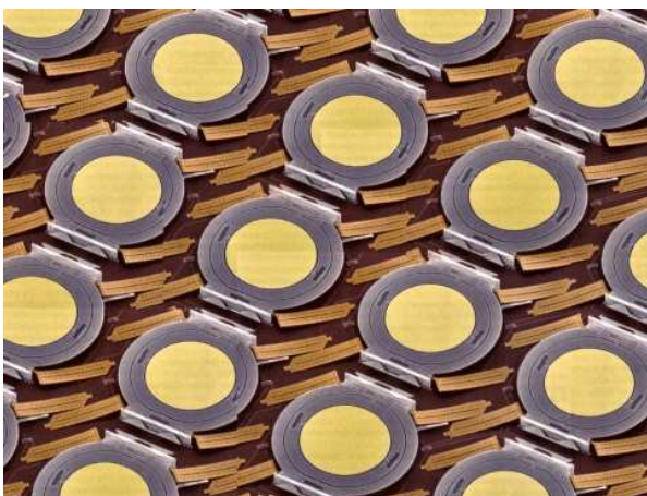
Figure 3. MEMS Microscopic Mirror Optical Switch Array
